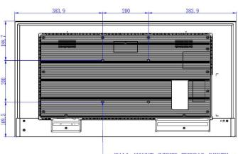
WALL MOUNT SCREW THREAD DEPTH: 4-M6x12mm
